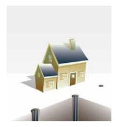
Protecting the deep earth environment with a proper grouting material is just as important as providing heat transfer between the piping system and the surrounding earth. Vertical loops are generally more expensive to install, but require less piping and less land area than horizontal loops.
